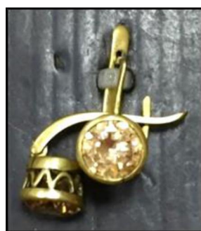
Fig. 6. Earrings with openwork casts and seam locks
