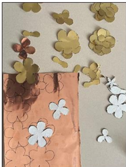
Fig. 1. Templates of metal blanks for “rose” petals
