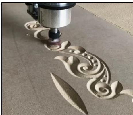
Fig. 9. Use of vector images (vector layouts) for NCP milling machines
