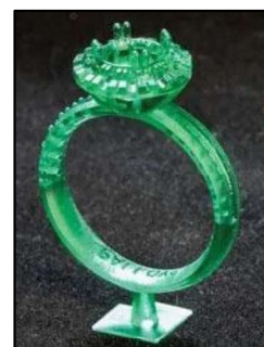
Fig. 8. Model of a jewelry item printed on a 3D printer
